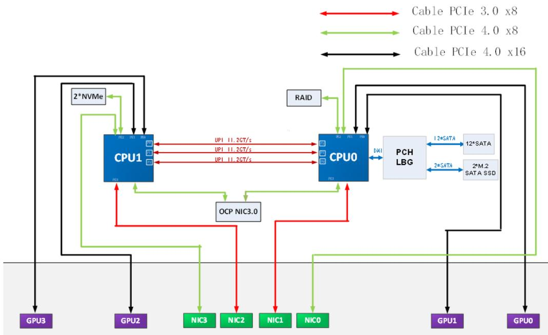
Figure 4-21 PCIe Topology Logic Block Diagram (Topology 2)
