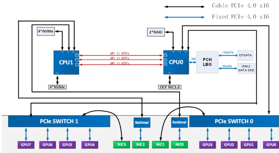
Figure 4-17 PCIe Topology Logic Block Diagram (Common GPU Topology/Multi-Host OCP NIC 3.0)
