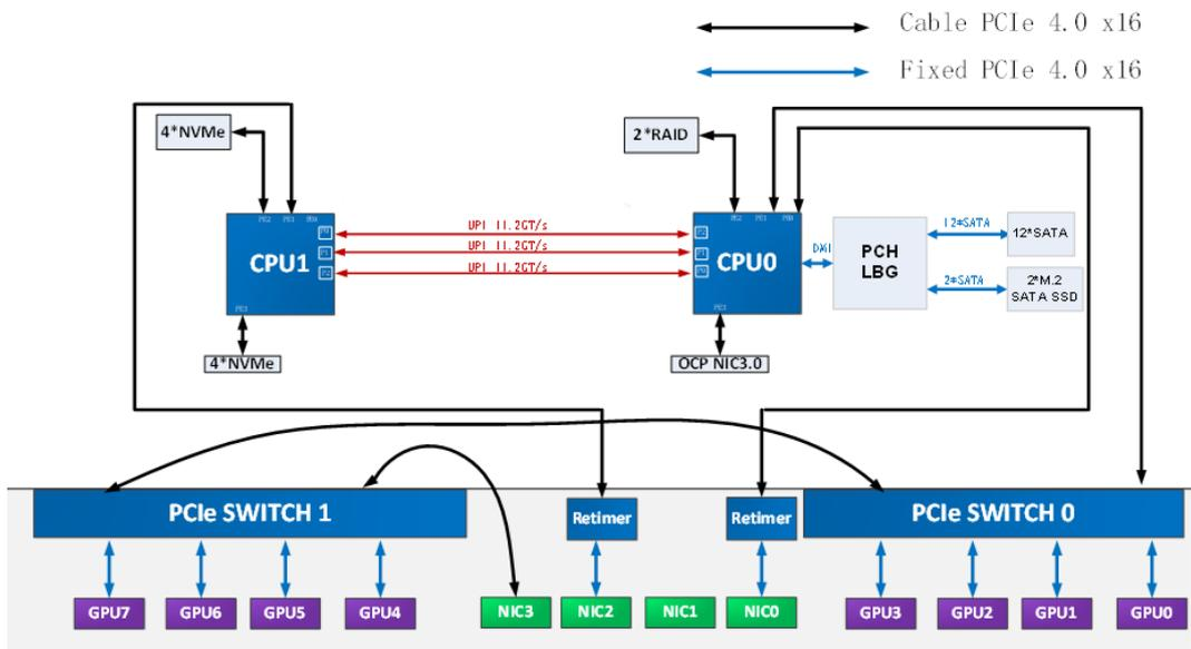
Figure 4-15 PCIe Topology Logic Block Diagram (Cascade GPU Topology/Multi-Host OCP NIC 3.0)
