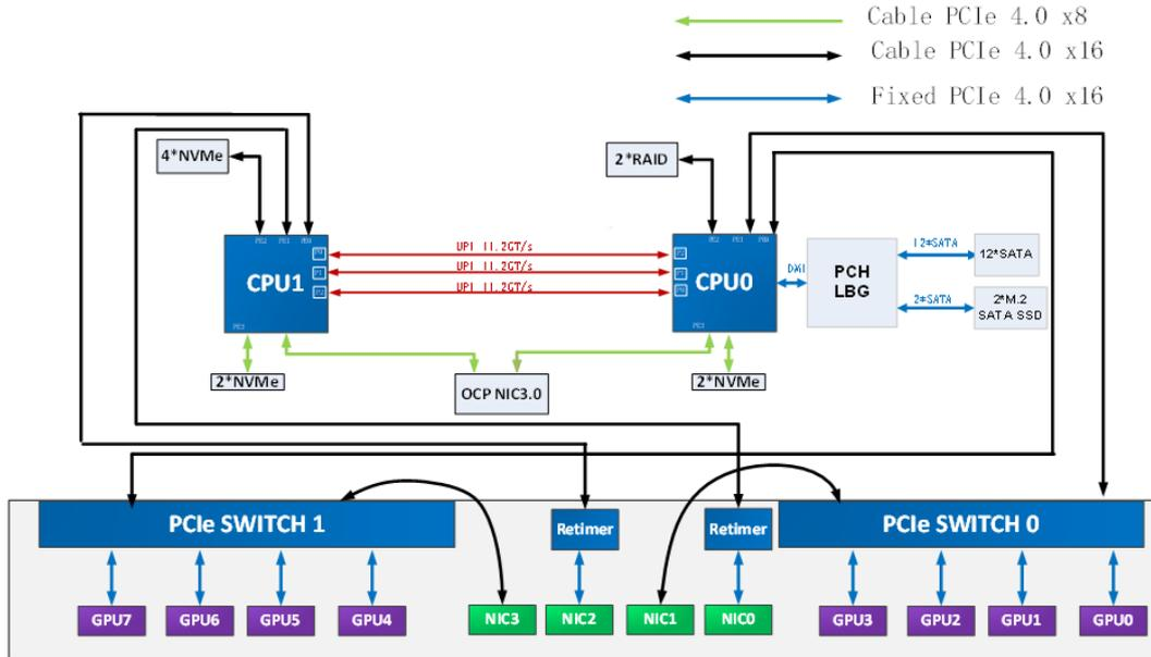
Figure 4-18 PCIe Topology Logic Block Diagram (Supporting N10X SmartNIC Topology)
