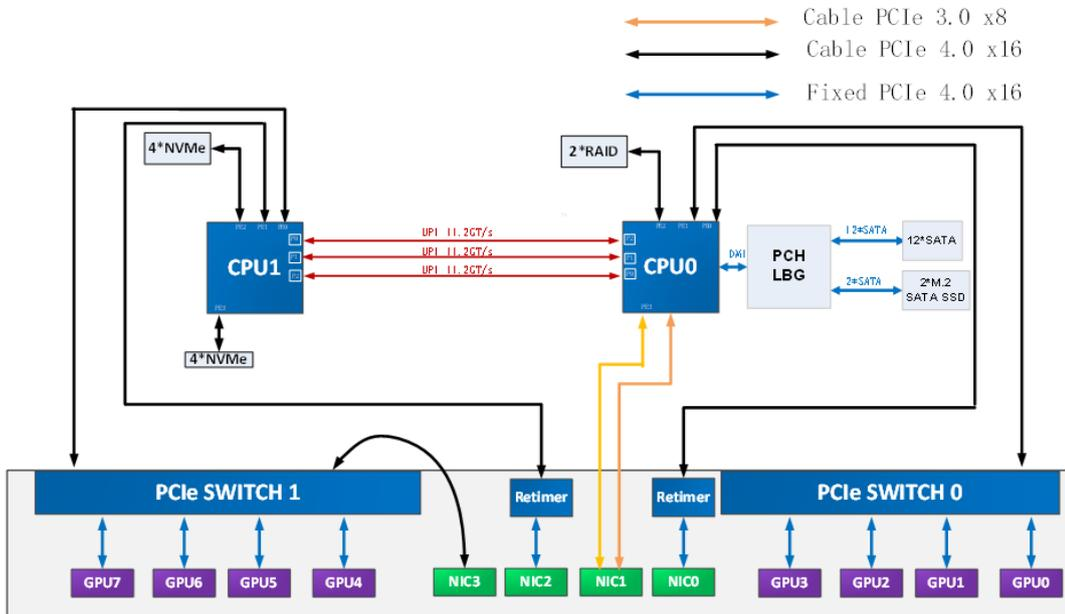
Figure 4-19 PCIe Topology Logic Block Diagram (Single-CPU Topology)
