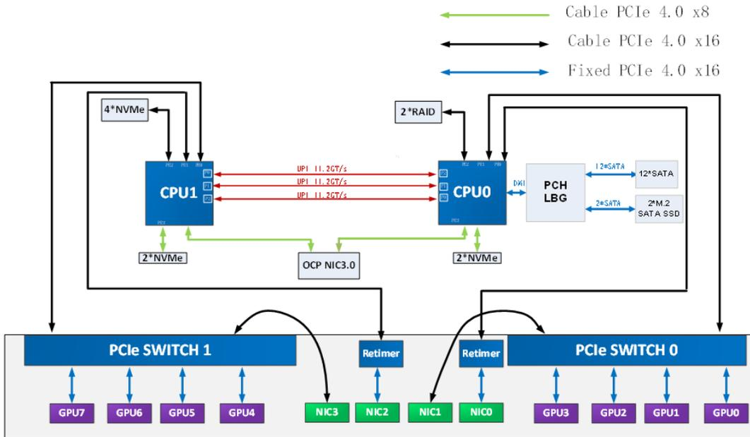
Figure 4-14 PCIe Topology Logic Block Diagram (Cascade GPU Topology/Single-Host OCP NIC 3.0)
