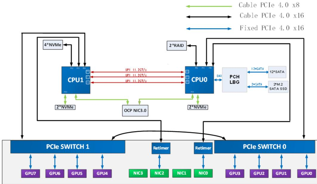
Figure 4-8 PCIe Topology Logic Block Diagram (Balance or Common GPU Topology/Single-Host OCP NIC 3.0)
