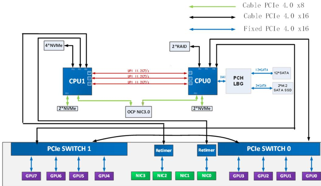
Figure 4-12 PCIe Topology Logic Block Diagram (Balance GPU Topology/Single-Host OCP NIC 3.0)
