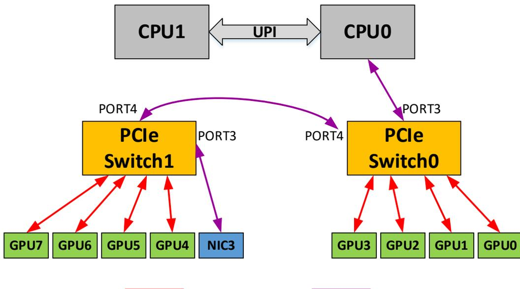
Features: Only CPU0 is connected to a PCIe switch and this PCIe switch interconnects with another one. Each PCIe switch is connected to 4 GPUs. The PCIe
