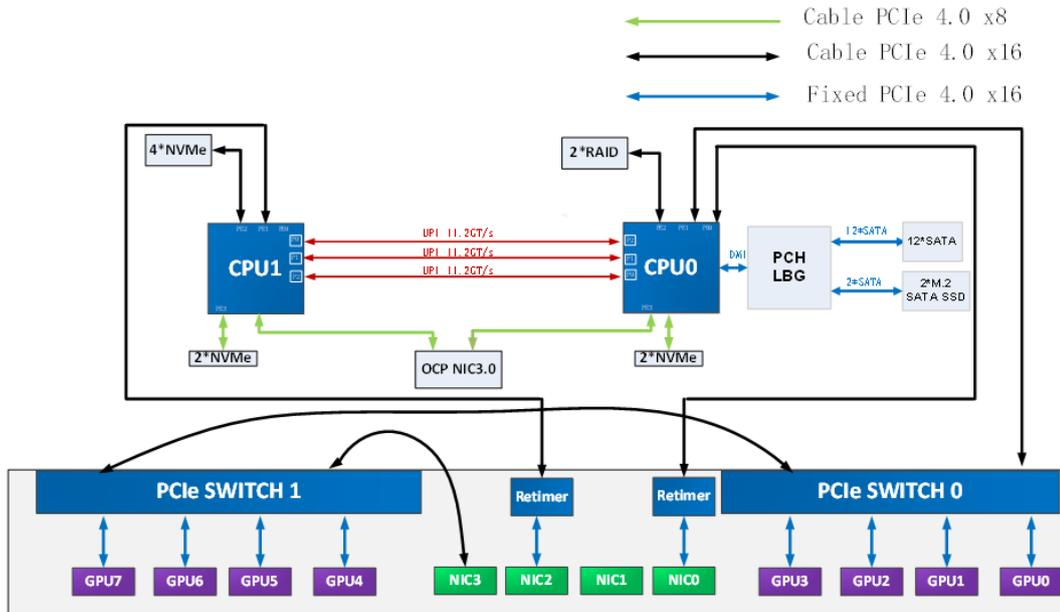
Figure 4-16 PCIe Topology Logic Block Diagram (Common GPU Topology/Single-Host OCP NIC 3.0)
