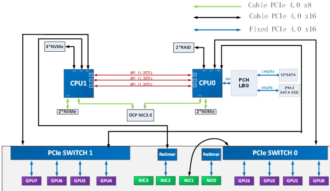
Figure 4-10 PCIe Topology Logic Block Diagram (Common or Cascade GPU Topology/Single-Host OCP NIC 3.0)
