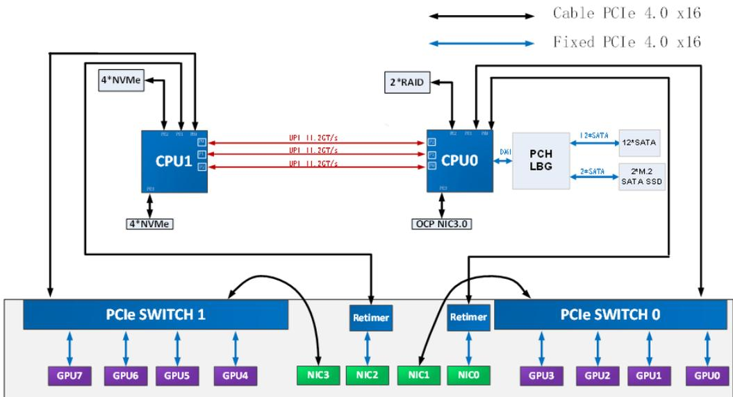
Figure 4-13 PCIe Topology Logic Block Diagram (Balance GPU Topology/Multi-Host OCP NIC 3.0)
