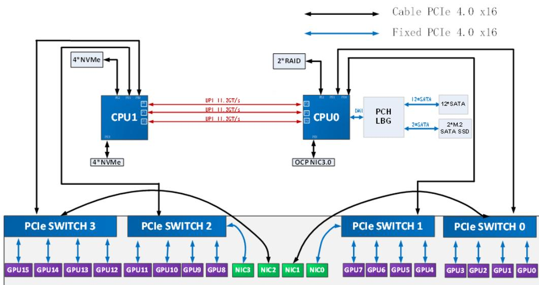
Figure 4-23 PCIe Topology Logic Block Diagram (PCIe 4.0 Switch/Multi-Host)
