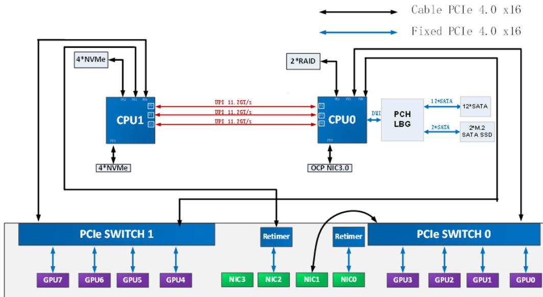
Figure 4-9 PCIe Topology Logic Block Diagram (Balance or Common GPU Topology/Multi-Host OCP NIC 3.0)
