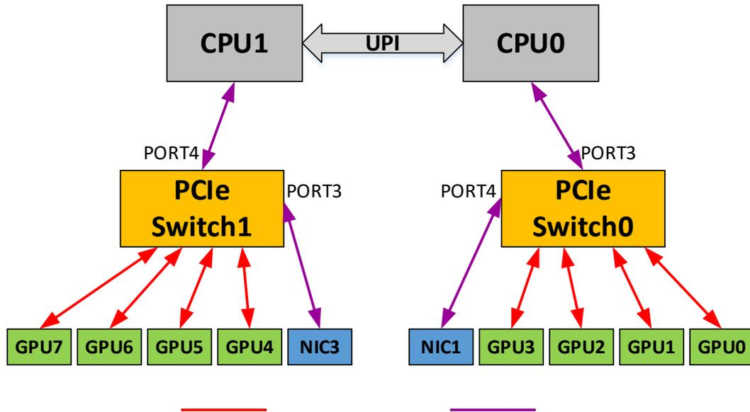
Features: Each CPU has a PCIe switch, which is then connected to 4 GPUs. This topology maximizes CPU utilization and provides a greater upstream bandwidth. But in this topology, the P2P communication between 2 GPUs connected to different CPUs is limited by the UPI link speed.
