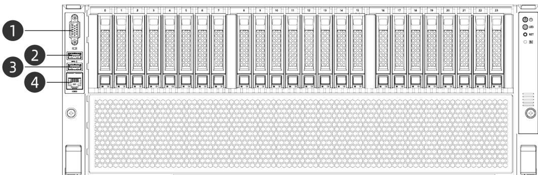
Figure 5-5 Front Panel Ports (12 × 3.5-inch Drive Configuration)
