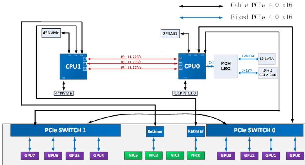
Figure 4-11 PCIe Topology Logic Block Diagram (Common or Cascade GPU Topology/Multi-Host OCP NIC 3.0)
