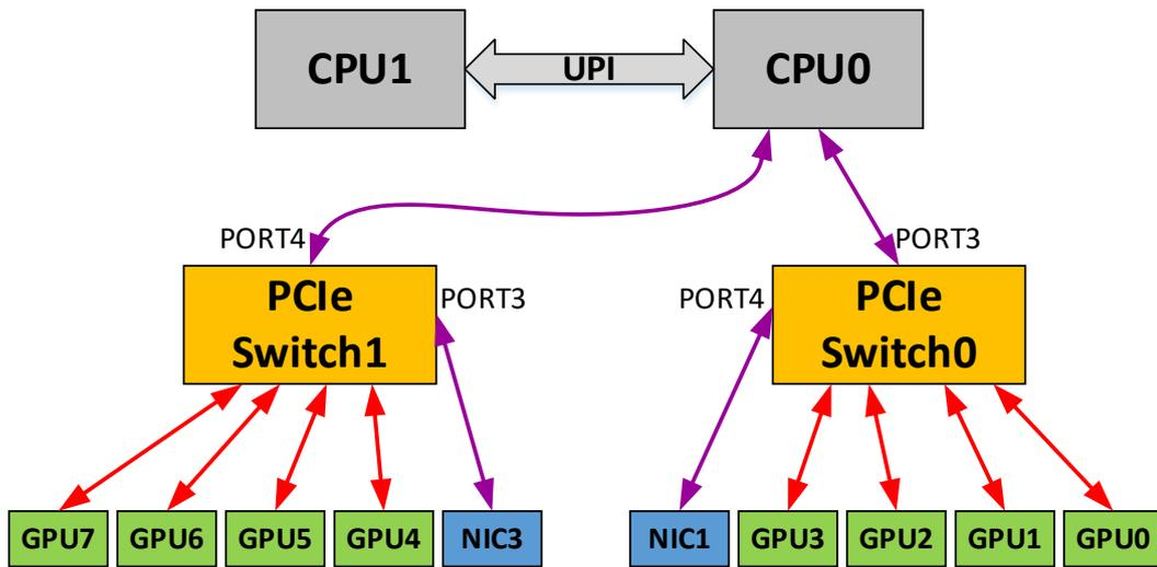
Features: CPU0 is connected to 2 PCIe switches. Each PCIe switch is connected to 4 GPUs. The communication between 2 GPUs connected to different PCIe switches can be accomplished without cross-CPU communication, delivering better P2P communication and higher data throughput.
